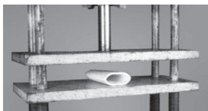
PVC conduit will stay compressed if it is crushed. (Same for steel conduit.)
